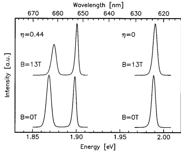
FIG. 1. PL spectra from a disordered sample (right-hand side) and an ordered sample ( $\eta=0.44$ , left-hand side), taken at zero magnetic field (bottom) and at 13 T (top). The spectra are normalized and shifted on the intensity axis.
