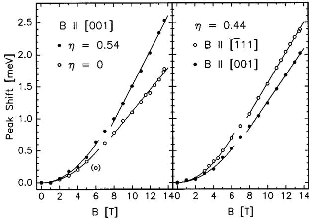
FIG. 2. Energy shift  $\delta E$  of the PL peak with increasing magnetic field. (a) Comparison of the disordered with the most ordered sample; (b) comparison of the peak shift with  $\mathbf{B}||[001]$  and with  $\mathbf{B}||[111]$ . Lines are fits to the data: For  $0 \text{ T} \leq B \leq 6$  T, a parabola ( $\delta E = a_1 B^2$ ) fits the data, whereas a linear magnetic shift ( $\delta E \propto a_2 B$ ) describes the data well for  $8 \text{ T} \leq B < 14$  T.
