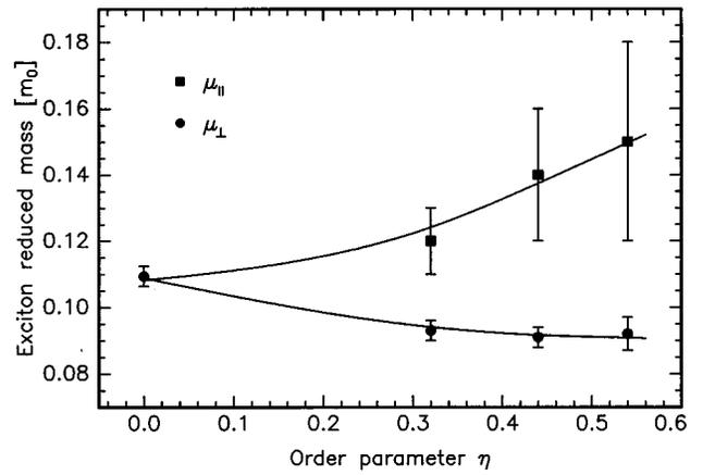
FIG. 3. Anisotropic exciton reduced masses as a function of order parameter  $\eta$ , derived from the experimentally determined diamagnetic shift of the excitonic PL transition.
