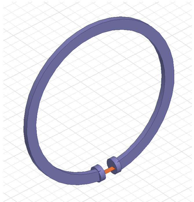
Fig. 8. SRR simulated with both ideal and non-ideal non-Foster loading.
