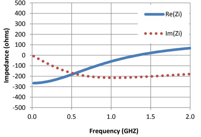
Fig. 3. Simulation results showing real part of  $Z_i$  (solid blue) and imaginary part of  $Z_i$  (dotted red).
