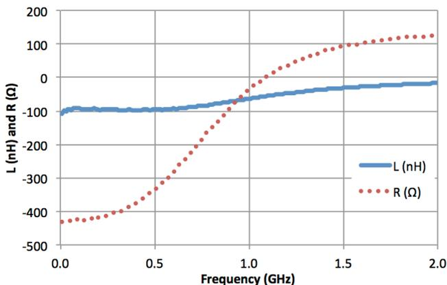
Fig. 6. Data for prototype circuit showing measured inductance L in nH (solid blue) and measured resistance R in ohms (dotted red).
