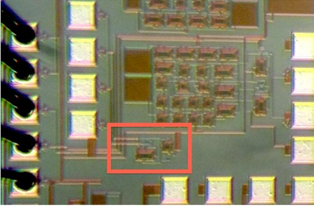
Fig. 5. Photograph of prototype negative inductance circuit with red box showing location of the circuit of Fig. 1.
