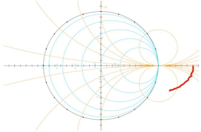
Fig. 7. Smith chart showing measured S11 of input impedance  $Z_i$ .
