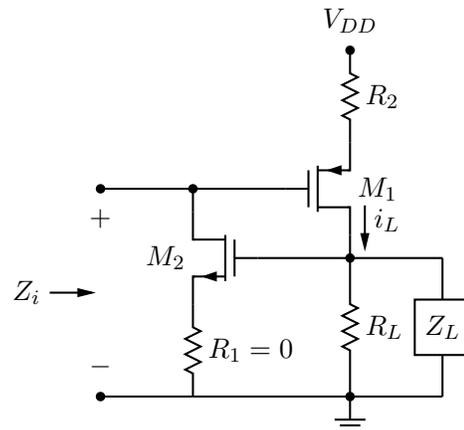
Fig. 1. Schematic of proposed CMOS negative inductance circuit.
