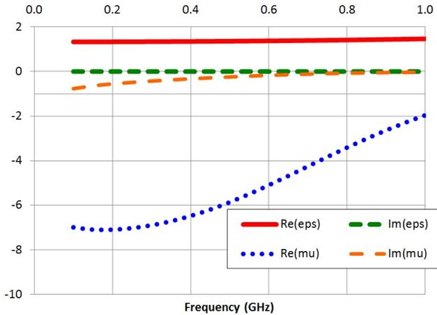
Fig. 9. Extracted real and imaginary parts of permeability and permittivity, for the ideal case where  $R=0$ .
