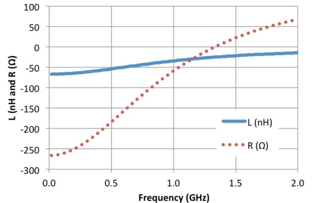
Fig. 4. Simulation results showing extracted inductance  $L$  in nH (solid blue) and resistance  $R$  in ohms (dotted red).
