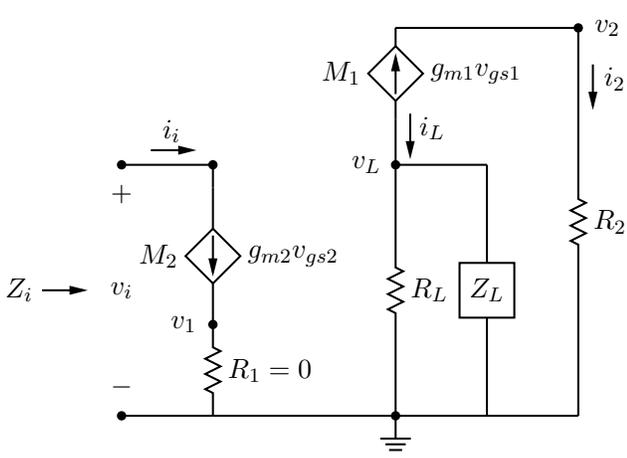
Fig. 2. Small-signal model.
