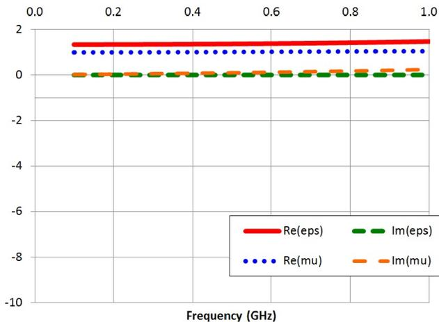
Fig. 10. Extracted real and imaginary parts of permeability and permittivity, for the real case where  $R = -240$   $\Omega$ .
