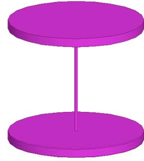
Fig. 2. Electric unit cell example showing example electric disk resonator (EDR) with two brass disks connected by a cylindrical rod. The outer faces of the two metal disks at the top and bottom of the structure have areas  $A_D$ , and are connected together by a metal post with inductance  $L_p$  and length  $l_p$ .
