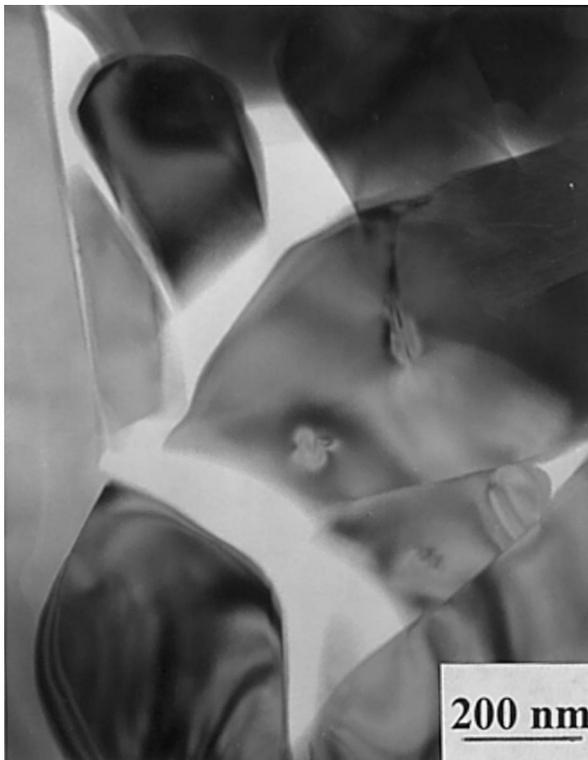
Fig. 1. TEM micrograph of GS44 ruptured after 3.95 h of creep at 1275°C under 80 MPa.
