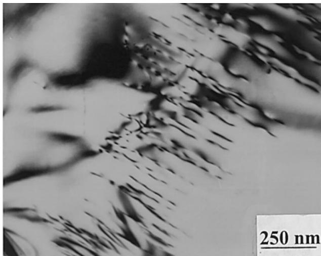
Fig. 6. Dislocation arrays in a silicon nitride grain of GS44 crept at 1275°C under 80 MPa.
