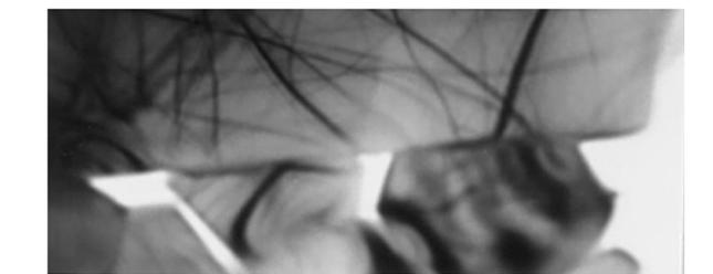
Fig. 4. TEM micrograph showing strain whorls at the grain boundaries (a) and a portion of the large angle convergent electron diffraction disk (b) from (a) showing severely bent Bragg lines close to the grain boundaries where the strain whorls lie.
