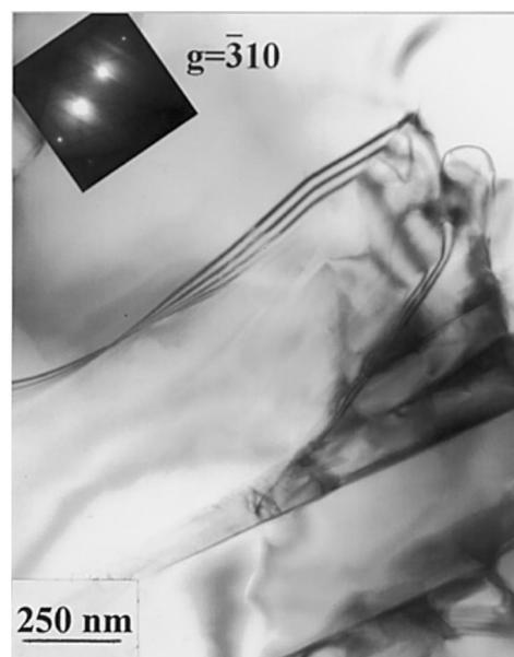
Fig. 10. Two beam condition bright field image showing dislocations out of contrast with the excited reflection being  $g = \bar{3}10$ .
