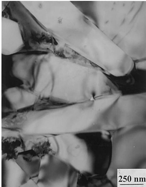
Fig. 3. TEM micrograph of GS44 crept at 1000°C under 80 MPa for 500 h without failure. It shows elongated grains and strain whorls of less population as compared to the sample crept at 1275°C.
