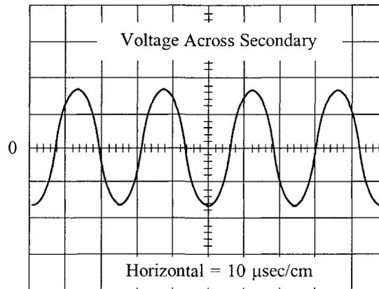
Figure 19-10. Current-fed Converter, Secondary Sine Wave Secondary Voltage.
