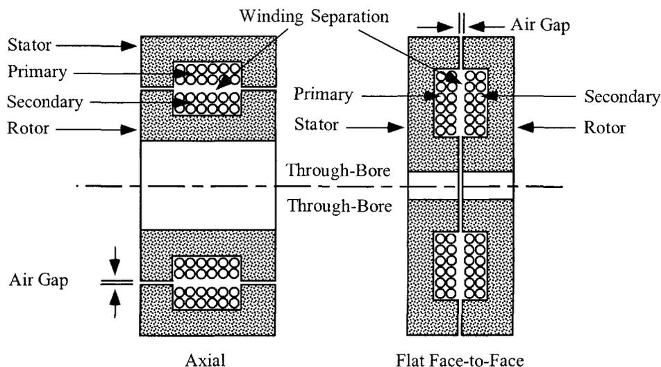
Figure 19-11. Geometries of the Basic Type Rotary Transformers.
