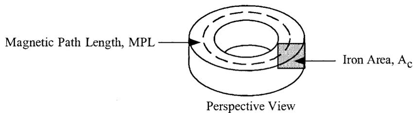
**Figure 19-12.** Typical Perspective View of a Toroidal Core.
