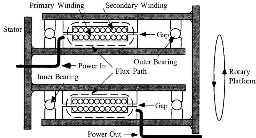
**Figure 19-2.** Pictorial of an Axial, type Rotary Transformer.
