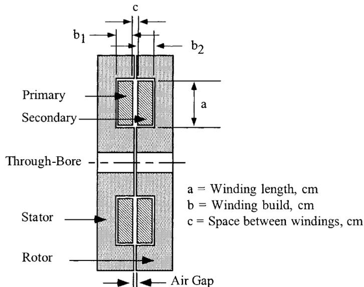
**Figure 19-7.** Flat Plane Rotary Transformer, Showing Winding Dimensions.
