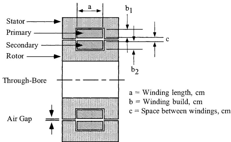
**Figure 19-6.** Axial Rotary Transformer, Showing Winding Dimensions.
