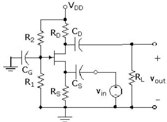
The ac small signal model for the CG amplifier is shown to the right (Note that the illustration given in Figure 6.37b of your text is incorrect.).
