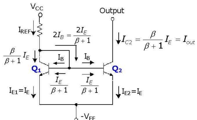
and emitters tied together. The transistor designated  $Q_1$  in the figure is connected as a diode by shorting its base and collector terminals.
