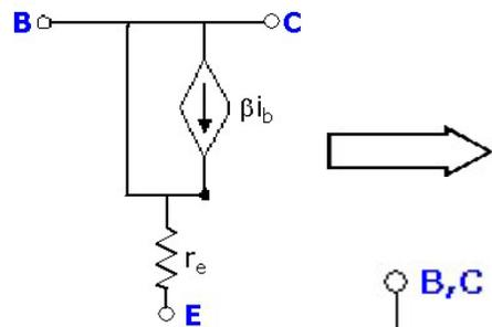
The dependent source is shorted out and we end up with a single resistance between the base-collector terminal and the emitter terminal.
