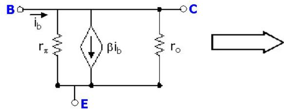
Assuming  $r_\pi \ll r_o$ ,  $r_\pi || r_o \approx r_\pi$  and the circuit is simplified to a single resistor in parallel with the dependent current source:
