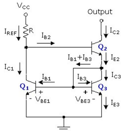
$$I_{E2} = I_{C3} + I_{B1} + I_{B3}. \quad (\text{Equation 5.71})$$
