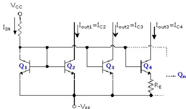
modified version of Figure 5.31 in your text. Note that  $Q_2$  and  $Q_3$  form a current mirror with transistor  $Q_1$ , while  $Q_4$  is a Widlar current source because it has a resistor in the emitter leg. The amount of current delivered by this source can be determined by the size of this emitter resistor. Also, when using the Widlar circuit, the output current(s) may be different from the original reference current,  $I_{IN}$ .
