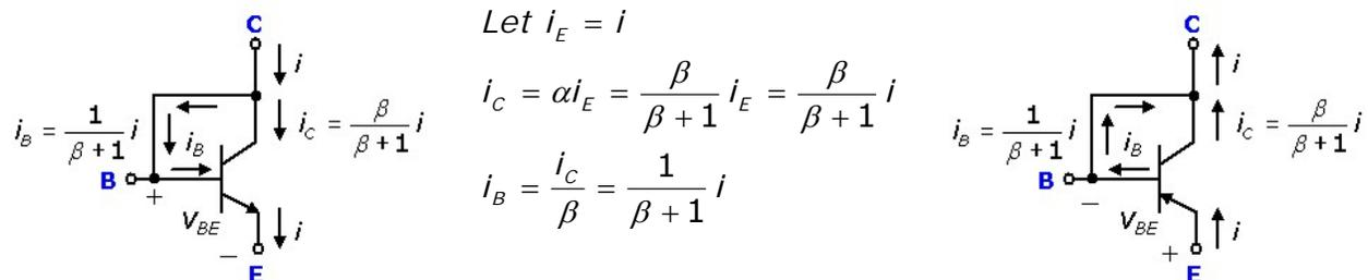
To illustrate the development of the simplified model for a diode-connected BJT, we're going to use the npn device. As usual, development for the pnp is directly analogous with current directions reversed and polarities switched.
