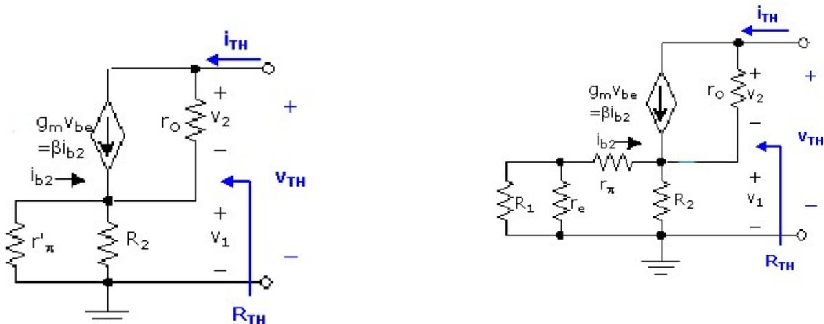
Using the method of applying a test voltage  $v_{TH}$  and solving for the resulting current  $i_{TH}$  (or vice versa), we can solve for  $R_{TH}=v_{TH}/i_{TH}$ . Analyzing the simplified circuit (above right), we get the following definitions:
