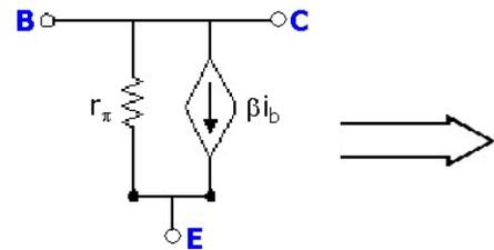
Now...reflecting  $r_\pi$  from the base circuit to the emitter circuit (recall that  $r_\pi = (\beta + 1)r_e$ ), we are left with a short in the base-emitter leg:
