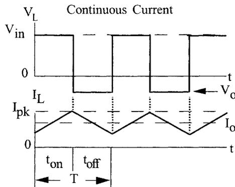
Figure 13-11. Continuous, Current Inverting, Buck-Boost Converter Waveforms.
