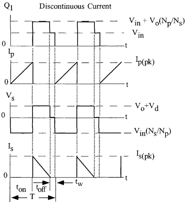
Figure 13-13. Discontinuous Current, Isolated, Buck-Boost Converter Waveforms.
