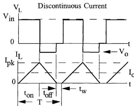
Figure 13-10. Discontinuous, Current Inverting, Buck-Boost Converter Waveforms.
