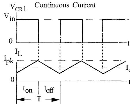
**Figure 13-5.** Continuous Current Buck Converter Waveforms.
