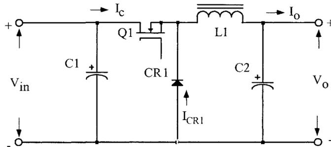
Figure 13-3. Schematic of a Buck Switching Converter.
