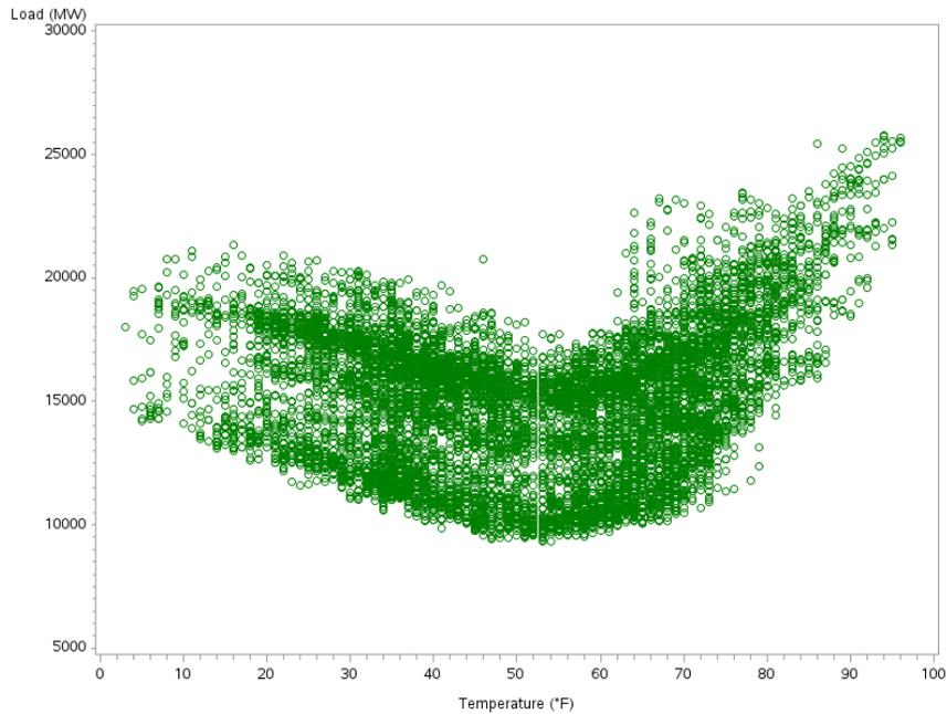
**Figure 2-2: Scatter plot for a typical load and temperature relationship**
