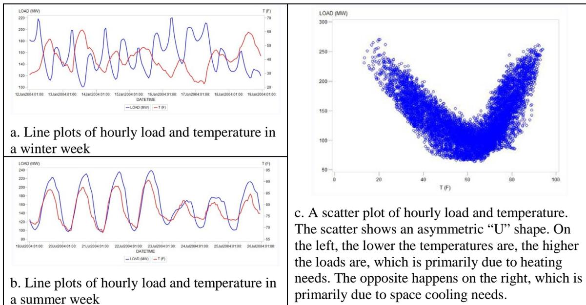
**Figure 1-1: Relationship between load and temperature**
