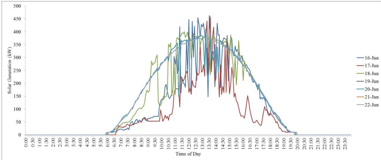
**Figure 1-4: One week of solar power generation at 5-minute interval**
