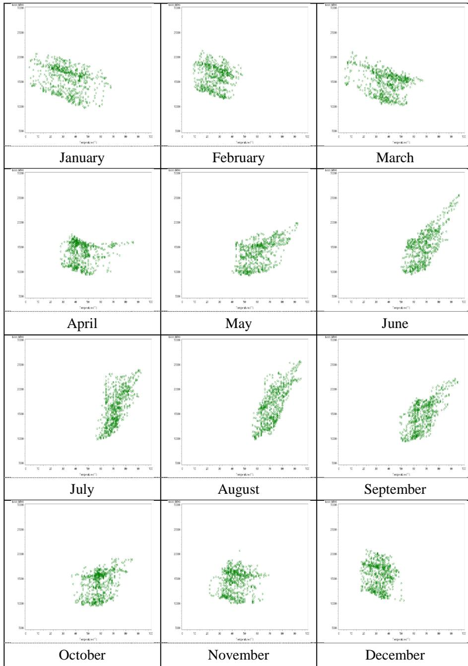
**Figure 2-5: Monthly scatter plots for a typical load and temperature relationship**
