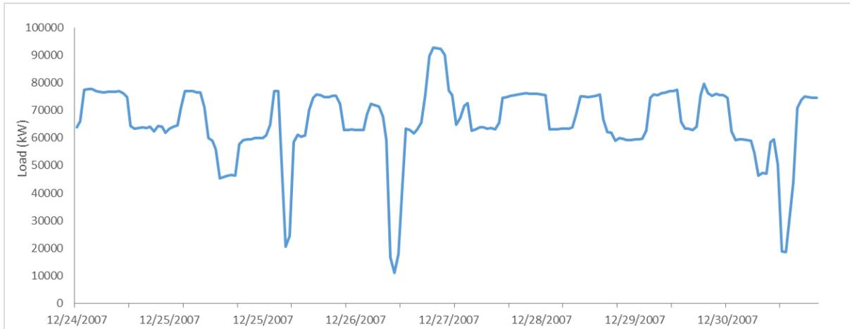
**Figure 3-3: Hourly load profile of an industrial customer**
